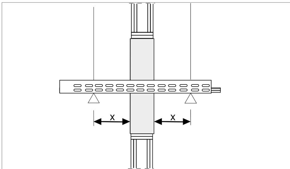
Fig. 3: Maximum distance for supports
