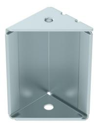
Additional Z support for the elevation of the walkable BKRS cable tray system on the floor. Fastening with flat-head screw FKS 6 x 12 mm (item no. 6049246).
