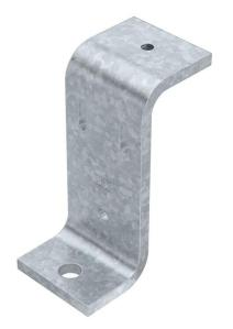
Z support as a stand-off of the walkable BKRS cable tray system on the floor. Fastening of the cable tray on the Z support with flat-head screw FKS 6 x 12 mm (item no. 6049246) with M6 threaded hole.
