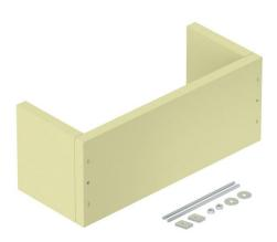
Strain relief as an effective support measure for vertical cable routing, according to DIN 4102 Part 12. Approved for all cable types and all vertical routing systems, which are mounted directly on solid walls. Maintenance of electrical function classes E30 to E90. Empty housing for individual filling with the PYROSIT® NG fire protection foam and/or PYROPLUG® Block insulation systems, incl. mounting set and labelling panel.
