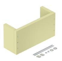
Strain relief as an effective support measure for vertical cable routing, according to DIN 4102 Part 12. Approved for all cable types and all vertical routing systems, which are mounted directly on solid walls. Maintenance of electrical function classes E30 to E90. Empty housing for individual filling with the PYROSIT® NG fire protection foam and/or PYROPLUG® Block insulation systems, incl. mounting set and labelling panel.
