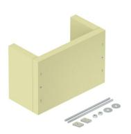
Strain relief as an effective support measure for vertical cable routing, according to DIN 4102 Part 12. Approved for all cable types and all vertical routing systems, which are mounted directly on solid walls. Maintenance of electrical function classes E30 to E90. Empty housing for individual filling with the PYROSIT® NG fire protection foam and/or PYROPLUG® Block insulation systems, incl. mounting set and labelling panel.
