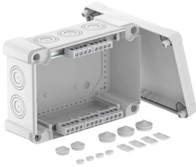
Junction box with terminal strip for the connection of cables and lines indoors and in outdoor areas. Rectangular design with knock-out entries. Suitable for wall and ceiling mounting with the option to fasten outside, inside or to mount via the corner domes. Particularly impact resistant with IK09. Cover with quick lock, sealable. Made from halogen-free and UV-resistant materials.
