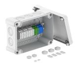
Junction box for the connection of cables and lines indoors and in outdoor areas. Rectangular design with knock-out entries. Suitable for wall and ceiling mounting with the option to fasten outside, inside or to mount via the corner domes. Particularly impact resistant with IK09. Cover with quick lock, sealable. Made from halogen-free and UV-resistant materials.
