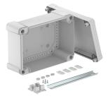
Junction box with hat profile rail for the connection of cables and lines indoors and in outdoor areas. Rectangular design without entries. Suitable for wall and ceiling mounting with the option to fasten outside, inside or to mount via the corner domes. Particularly impact resistant with IK09. Cover with quick lock, sealable. Made from halogen-free and UV-resistant materials.
