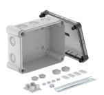
Junction box with hat profile rail for the connection of cables and lines indoors and in outdoor areas. Rectangular design with knock-out entries. Suitable for wall and ceiling mounting with the option to fasten outside, inside or to mount via the corner domes. Particularly impact resistant with IK09. Transparent cover with quick lock, sealable. Made from halogen-free and UV-resistant materials.
