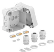
Junction box with terminal for the connection of cables in indoor and outdoor areas. Square design with knock-out entries. Suitable for wall and ceiling mounting with the option to fasten outside, inside or to mount via the corner domes. Particularly impact resistant with IK09. Cover with quick lock, sealable. Made from halogen-free and UV-resistant materials.
