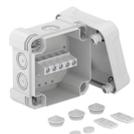
Junction box with terminal strip for the connection of cables and lines indoors and in outdoor areas. Square design with knock-out entries. Suitable for wall and ceiling mounting with the option to fasten outside, inside or to mount via the corner domes. Particularly impact resistant with IK09. Cover with quick lock, sealable. Made from halogen-free and UV-resistant materials.
