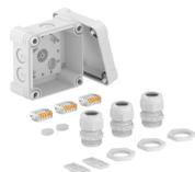
Junction box with terminal for the connection of cables and lines indoors and in outdoor areas. Square design with knock-out entries. Suitable for wall and ceiling mounting with the option to fasten outside, inside or to mount via the corner domes. Particularly impact resistant with IK09. Cover with quick lock, sealable. Made from halogen-free and UV-resistant materials.
