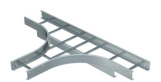
Horizontal T branch piece, for all wide span cable ladders of 110 mm side height. For further stabilisation, additional supports should be planned for the area of the fittings.
