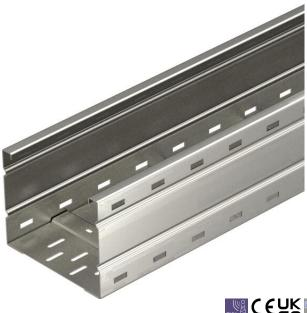
Wide span cable tray system, perforated, with a side height of 160 mm. Straight connectors of type WRVL 160 should be ordered separately and in the appropriate quantity. Magnetic shield insulation without cover 20 dB, with cover 50 dB.
