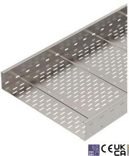
Wide span cable tray system, perforated, with a side height of 110 mm. Straight connectors of type WRVL 110 should be ordered separately and in the appropriate quantity. Magnetic shield insulation without cover 20 dB, with cover 50 dB.
