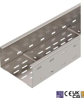
Wide span cable tray system, perforated, with a side height of 110 mm. Straight connectors of type WRVL 110 should be ordered separately and in the appropriate quantity. Magnetic shield insulation without cover 20 dB, with cover 50 dB.
