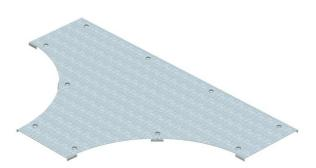
Cover for wide span T branch piece with pre-mounted turn buckles. As the connector is mounted from the outside, the fitting cover is 300 mm shorter than the corresponding fitting. This must be considered when installing the track elements.
