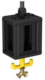
Empty housing with 1 m pipe 1/2" and connection for compressed air hose 13 x 3.5 mm and 2-way distributor 1/2". With suspension lug and grip hook, for the installation of electrical resources, with included partition. Without cover plates to supply workplaces in wet areas. Protection rating: IP44.
