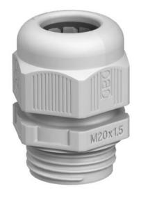
The quickest and most convenient way of providing strain relief and tightness with cable glands on junction boxes and housings is with the tried-and-trusted V-TEC VM cable glands from OBO. With the integrated sealing lip and the special OBO lamella technology, protection class IP68 is achieved. Strain relief and tightness have been tested to DIN EN 62444.
