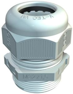
The quickest and most convenient way of providing strain relief and tightness with cable glands on junction boxes and housings is with the tried-and-trusted V-TEC VM cable glands from OBO. With the integrated sealing lip and the special OBO lamella technology, protection class IP68 is achieved. Strain relief and tightness have been tested to DIN EN 62444.
