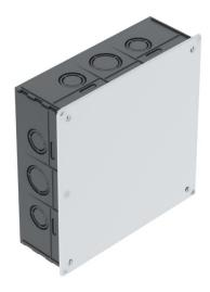
Flush-mounted connection box for clamping terminals, for use in masonry with an installation depth of at least 65 mm. With cover and cover screws (15 mm). Flat cover edge, roughened surface.
