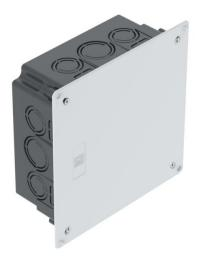
Flush-mounted connection box for clamping terminals, for use in masonry with an installation depth of at least 65 mm. With cover and cover screws (15 mm). Flat cover edge, roughened surface.
