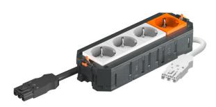
The ready-for-connection UTC4 universal support has 3 pre-installed 33° protective contact sockets in white and one pre-installed 33° protective contact socket in orange, 250 V $\sim$ , 16 A. With halogen-free connection cable. Suitable for VL connection cables and device installation units of nominal size R7, R9 and 9.
