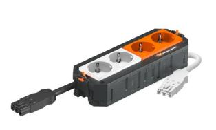
The ready-for-connection UTC4 universal support possesses 2 pre-installed 33° protective contact sockets in white and 2 pre-installed 33° protective contact sockets in orange (with surge protection module, type 3, according to DIN EN 61643-11), 250 V~, 16 A. Suitable for VL connection cables and device installation units of nominal size R7, R9 and 9.
