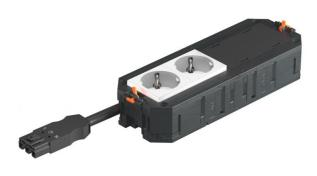
The ready-for-connection UTC4 universal support has 2 pre-installed 33° protective contact sockets in white and 2 blanking covers for retroinstallation of 2 installation devices of the Modul 45 series. Suitable for VL connection cables and device installation units of nominal size R7, R9 and 9.
