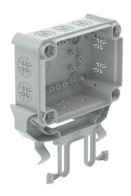
Pluggable lower part of junction box with universal fastening element for mounting on cable trays Unequipped, without cover. Halogen-free material and UV-resistant. Flame-resistant to DIN EN 60695/2/11, test temperature 650 °C. Impact resistance IK07 at room temperature. Protection class IP30.
