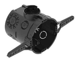
Flush-mounted device box with nail straps, for use in masonry with an installation depth of at least 66 mm.
