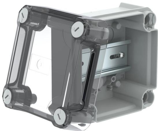
Closed junction box for the connection of cables and lines indoors and in protected outdoor areas. Square design without entries. Suitable for wall and ceiling mounting and on mounting panels. With the option to fasten inside and to mount via the corner domes. High, transparent cover with quick lock, sealable. Made from halogen-free and UV-resistant materials.
