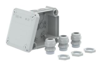
Junction box for the connection of cables and lines indoors and in protected outdoor areas. Square design with knock-out entries to the sides and knock-out entries in the bottom. Suitable for wall and ceiling mounting and on mounting panels. With the option to fasten inside and to mount via the corner domes. Cover with quick lock, sealable. Made from halogen-free and UV-resistant materials.
