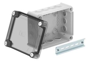
Junction box for the connection of cables and lines indoors and in protected outdoor areas. Rectangular design with plug-in seals to the sides and knock-out entries in the bottom. Suitable for wall and ceiling mounting and on mounting panels. With the option to fasten inside and to mount via the corner domes. High, transparent cover with quick lock, sealable. Made from halogen-free and UV-resistant materials.
