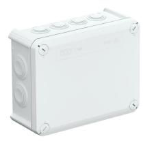
Junction box for the connection of cables and lines indoors and in protected outdoor areas. Rectangular design with plug-in seals to the sides and knock-out entries in the bottom. Suitable for wall and ceiling mounting and on mounting panels. With the option to fasten inside and to mount via the corner domes. Cover with quick lock, sealable. Flame-resistant type made from special polypropylene.
