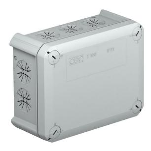
Junction box with strain relief entries for the connection of cables indoors and in protected outdoor areas. Rectangular design with knock-out entries to the sides and knock-out entries in the bottom. Suitable for wall and ceiling mounting and on mounting panels. With the option of fastening inside and to mount via the corner domes. Cover with quick lock, sealable. Made from halogen-free and UV-resistant materials.
