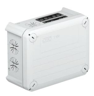
Junction box with Wieland sockets, 6s3p 3x2, for the connection of cables indoors and in protected outdoor areas. Rectangular design with knock-out entries to the sides and knock-out entries in the bottom. Suitable for wall and ceiling mounting and on mounting panels. With the option of fastening inside and to mount via the corner domes. Cover with quick lock, sealable. Made from halogen-free and UV-resistant materials.
