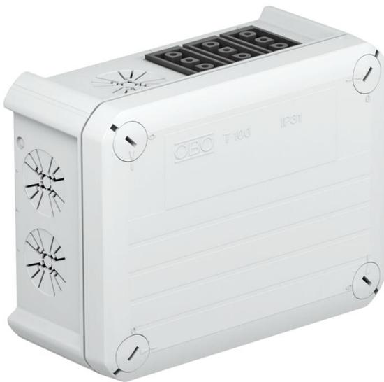
Junction box with Wieland sockets, 2s3p, for the connection of cables indoors and in protected outdoor areas. Rectangular design with knock-out entries to the sides and knock-out entries in the bottom. Suitable for wall and ceiling mounting and on mounting panels. With the option of fastening inside and to mount via the corner domes. Cover with quick lock, sealable. Made from halogen-free and UV-resistant materials.
