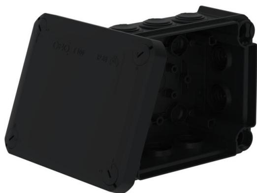
Junction box for the connection of cables and lines indoors and in protected outdoor areas. Rectangular design with plug-in seals to the sides and knock-out entries in the bottom. Suitable for wall and ceiling mounting and on mounting panels. With the option to fasten inside and to mount via the corner domes. Cover with quick lock, sealable. Made from halogen-free and UV-resistant materials.
