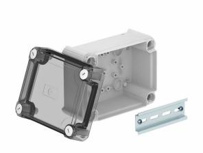
Closed junction box for the connection of cables and lines indoors and in protected outdoor areas. Rectangular design without entries. Suitable for wall and ceiling mounting and on mounting panels. With the option to fasten inside and to mount via the corner domes. High, transparent cover with quick lock, sealable. Made from halogen-free and UV-resistentant materials.
