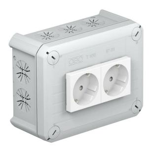
Junction box for the connection of cables indoors and in protected outdoor areas. Rectangular design with knock-out entries to the sides and knock-out entries in the bottom. Suitable for wall and ceiling mounting and on mounting panels. With the option of fastening inside and to mount via the corner domes. Cover with quick lock, sealable with retainer and 2 Modul 45 sockets. Made from halogenfree and UV-resistant materials.
