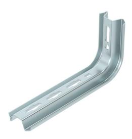
TP profile for use as lightweight support on horizontal concrete ceilings, on length 145–645 mm. Up to length 345 mm, the profile is used as a lightweight wall and support bracket.
