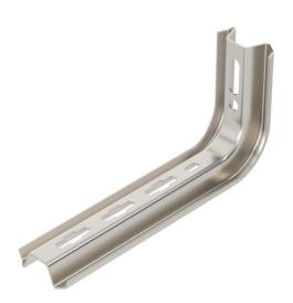
TP support / bracket for the fastening to horizontal concrete ceilings and walls. If the profile is fastened directly to the ceiling or the profile is screwed together as head reinforcement, then, for reasons of stability, always use the spacer, type DS 4.
