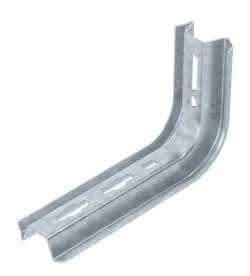
TP support/bracket for fastening to horizontal concrete ceilings and walls. If the profile is fastened directly to the ceiling or the profile is screwed together as head reinforcement, then, for reasons of stability, always use the spacer, type DS 4.
