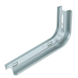
TP bracket with clamping lugs for screwless mesh cable tray fastening. If the bracket is fastened directly to the wall or the profiles are screwed together, then, for reasons of stability, always use the spacer, type DS 4. Mesh cable trays with a 50 x 100 mm grid width, e.g. type GRL, GR and GRM, can be fastened to the TP bracket without screws.
