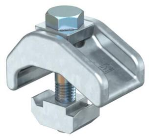
Heavy-duty chuck jaw with slide nut for fastening profile rails to steel girders. The clamping range of the chuck jaw is limited to the maximum fastening thickness. 30 mm.
