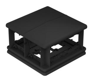
Raised-height installation unit for the installation of eight individual accessories with a support ring or support bracket on four sides. The current types (4 + 4) are separated using a partition. When multiple accessories are used, the connection capacity can be increased. Screw fixing groove for accessories: 60 mm, vertical.
