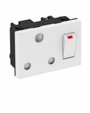
Socket, single 0°, with switch, South Africa/India, conforming to BS 546, with increased touch protection, with screw terminals, 2-pin, 16 A, 250 V~.
