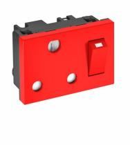
Socket, single 0°, with switch, South Africa/India, encoded version, conforming to BS 546, with increased touch protection, with screw terminals, 2-pin, 16 A, 250 V~.
