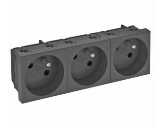
Socket with earthing pin Triple 33°, with increased touch protection, with screwless terminals, 2-pin, 16 A, 250V  $\sim$ , with connection terminals to IEC 60884-1.
