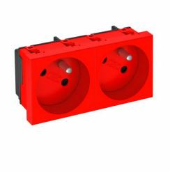
Socket with earthing pin Double 33°, with increased touch protection, with screwless terminals, 2-pin, 16 A, 250V  $\sim$ , with connection terminals to IEC 60884-1.
