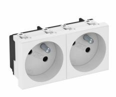
Socket with earthing pin Double 33°, with increased touch protection, with screwless terminals, 2-pin, 16 A, 250V  $\sim$ , with connection terminals to IEC 60884-1.
