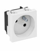
Socket with earthing pin Single 33°, with increased touch protection, with screwless terminals, 2-pin, 16 A, 250V  $\sim$ , with connection terminals to IEC 60884-1.
